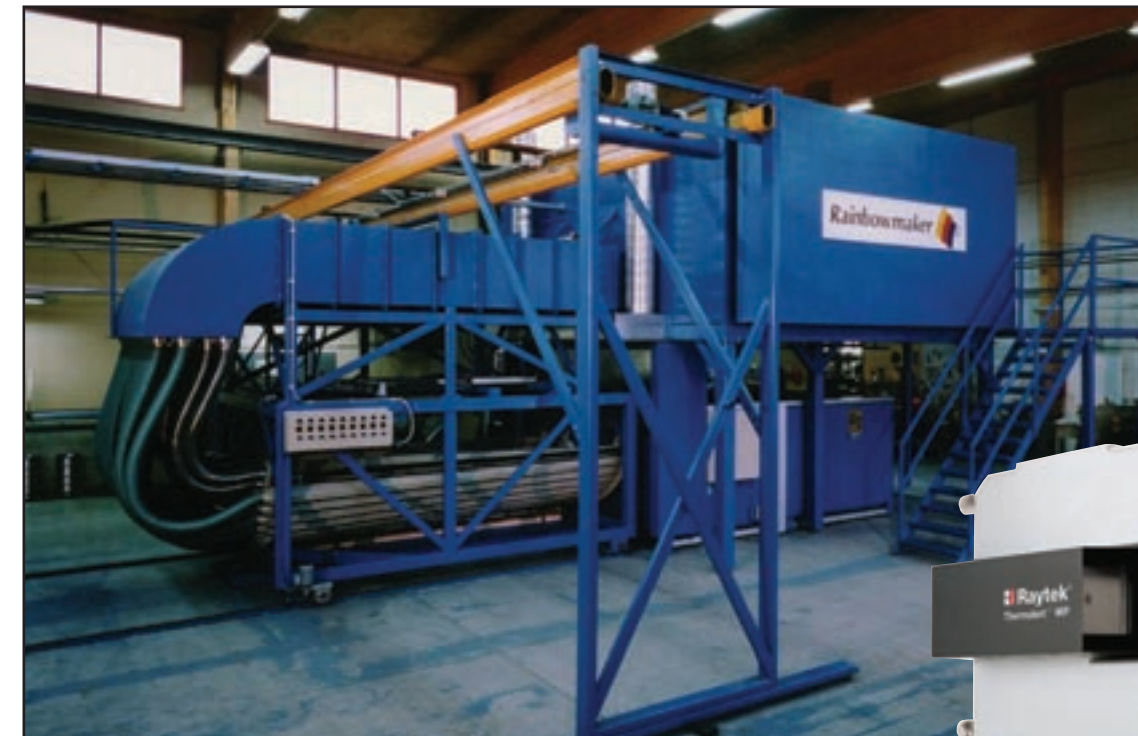
The GS100 provides real time temperature analysis for glass bending processes (Photo: Courtesy of Glassrobots OY, Tampere, Finland)
